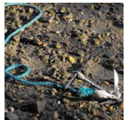
Step 7: Shows carabina for easy removal of spare anchor. Yes OK 'spare anchor' in a smackboat.
