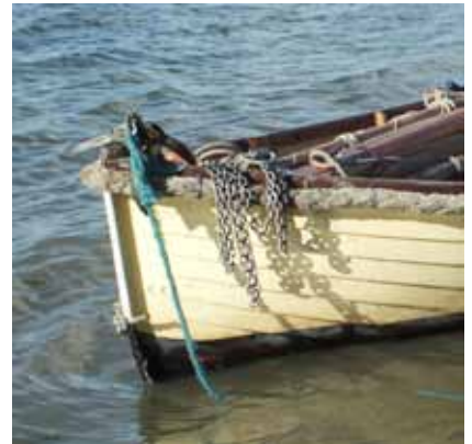
Step 1. Flake the anchor chain onto the gunwale with the anchor positioned such that it only just wants to stay with the boat.
