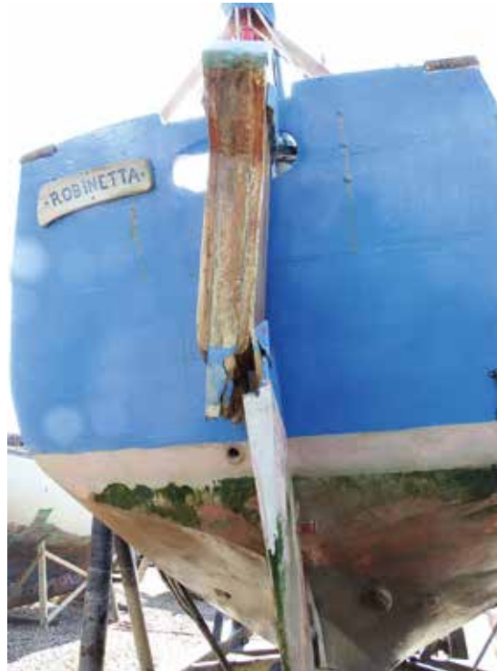
Robinetta's damaged rudder. Photograph by Alison Cable.
