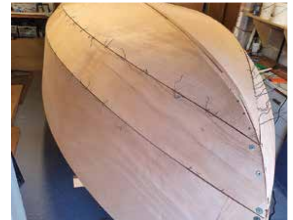
Hull panels stitched. Photo by Keith Mcllwain.
