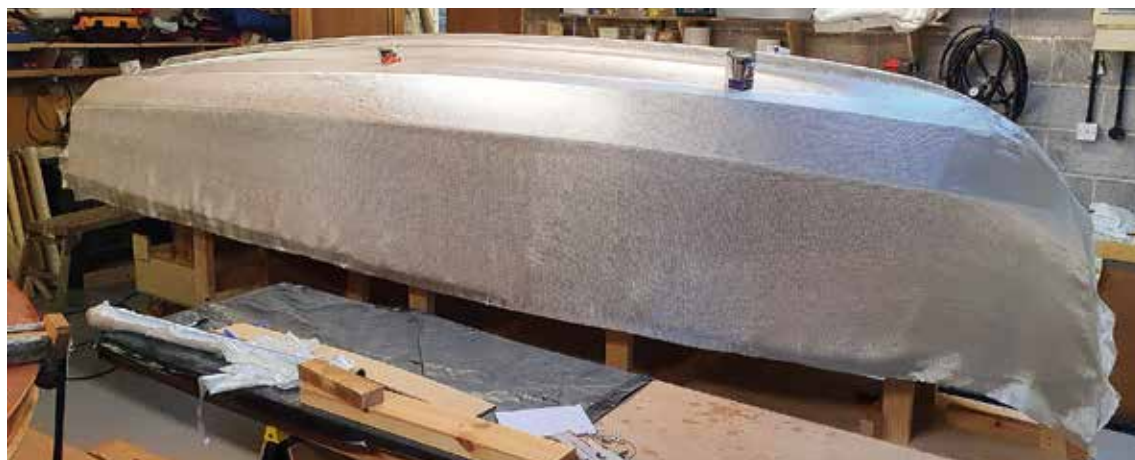
Hull being sheathed. Photo by Keith McIlwain.
