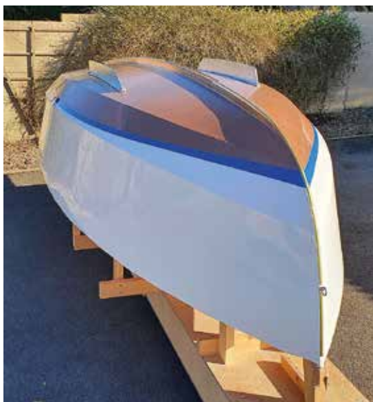
Hull finished prior to turning. Photo by Keith McIlwain.
