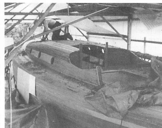
Cleaning off coach roof planking.
